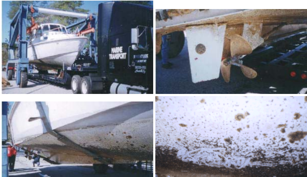
NRL Duplex Coating System (J501 Tiecoat + GE 1154 Topcoat) on USCG UTB Note: Fouling Easily Wiped Off by Hand (Bottom Right Photograph)
