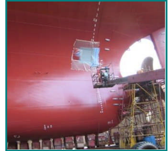
Aft-ship test patch - 3' x 3'
