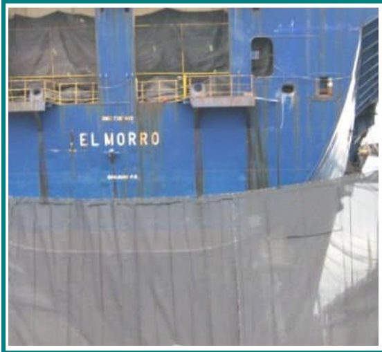
Drydock tarped for painting
