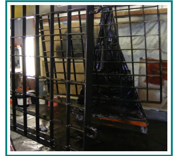
Completed silicone Surface Coat
